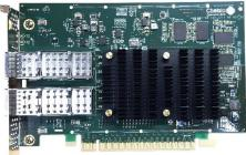
T62100-CR provides sub micro-second end-to-end latency, while offloading the host CPU from a variety of typical storage, networking, and cloud related protocols. Being a full height adapter, T62100-CR can accommodate more external memory modules on the card and hence specifically enhance the iSCSI performance on the target side. This enables savings in host CPU acquisition costs, power and operational costs, and dramatically increases iSCSI storage system performance.
