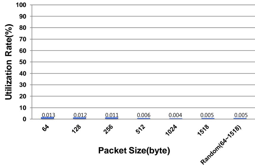
The performance result of 8 channels load balancing without non-block and its CPU utilization.
