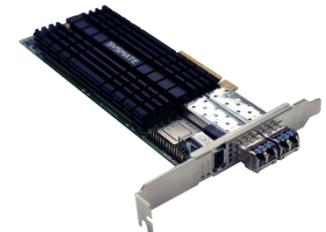
•IS4322C 2port 10Gbps Ethernet Packet Capture Network Adapter FPGA based
