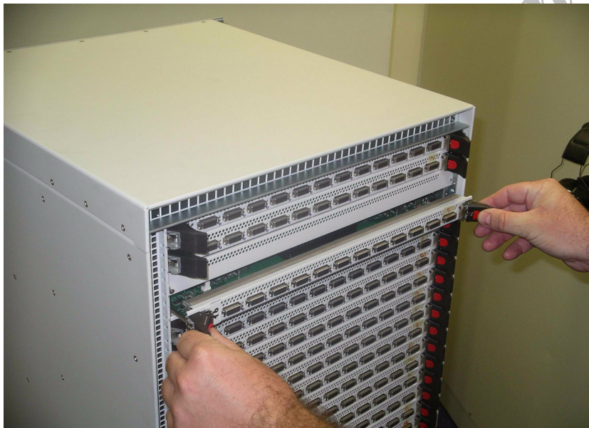
(a) Pressing the red buttons unlocks the ejectors
